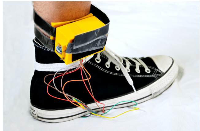
Figure 2: VRsneaky prototype: Raspberry Pi Zero W control unit mounted on a participant's leg. Force-sensing resistors (FSRs) used for gait awareness were placed under the shoe.
